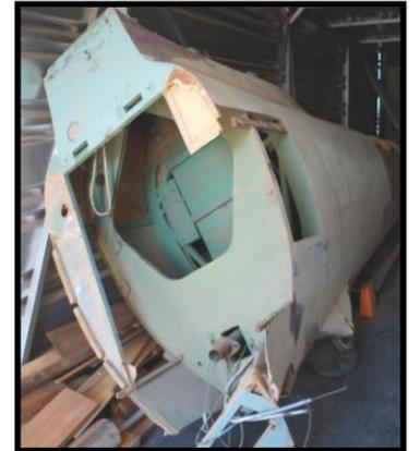
This altitude flight (a record) was the first of three incidents that resulted in extensive damage to the Gull 4. The second was after the ownership of the glider had passed to J.M. and W.P. Iggulden, Victorian Motorless Flight Group. It spun off a winch launch and crashed at Berwick. The third instance occurred at Bacchus Marsh when the pilot also lost control while being winch launched.
