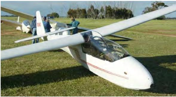
**\*Kaiser Ka-7 –VH-GNX** – A 16 metre two place sailplane, this aircraft has a steel tube fuselage whilst the wings and tailplane are constructed of wood. This has also been a very popular sailplane. **Donated by Bendigo Gliding Club.**
